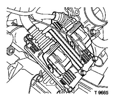
Wiring harness connector to intake manifold absolute pressure sensor.
