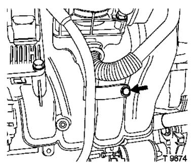
Cover with intake lines to air cleaner housing – clips
