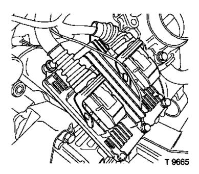
Wiring harness connector from injectors.
