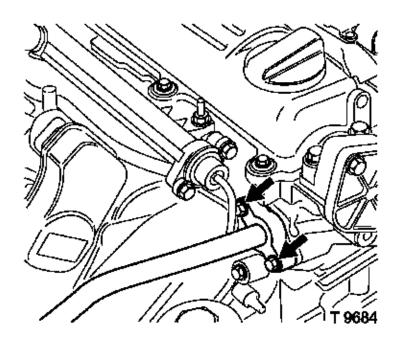
Guide tube to intake manifold – bolt (arrow) **10 Nm**.
