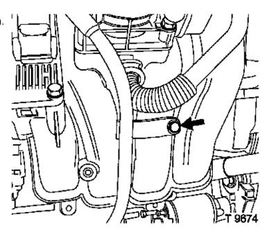
Exhaust gas recirculation line from cylinder head – bolts (arrow).
